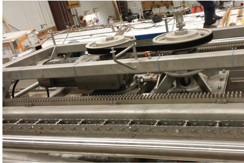
The 21-foot populated cable chain LAPP made for this finishing vat features two ÖLFLEX® FD VFD cables and one ÖLFLEX® ROBUST FD cable.
